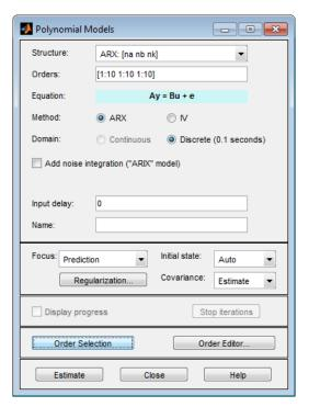
3 Click **Estimate** to open the ARX Model Structure Selection window, which displays the model performance for each combination of model parameters. The following figure shows an example plot.
